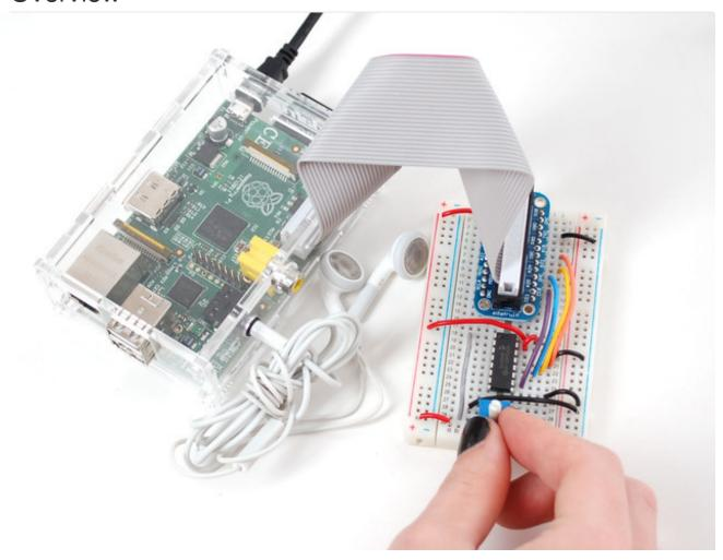
Teaching the Raspberry Pi how to read analog inputs is easier than you think! The Pi does not include a hardware analog-to-digital converter (http://adafru.it/eYp), but an external ADC (such as the MCP3008 (http://adafru.it/856)) can be used, along with some bit banged SPI code in Python to read external analog devices.
